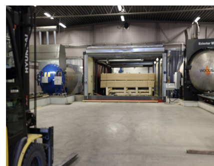
Photo: Woodsafe PRO and Woodsafe Exterior WFX vacuum pressure treatment plant.
