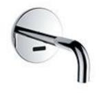
Concealed basin tap, with electronic control, for connection to cold or mixed water, projection 175 mm, fixed spout, battery operated (6V) / mains operated (230V), with Bluetooth adapter
