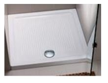
Antislip is a surface treatment which is applied to glazed and enamelled surfaces and then fired on and is thus optimally integrated into the surface structure. The surface offers a secure grip and is also easy to clean, and resistant to acids and scratching. Antislip has been tested against the German industrial standard DIN 51097 and offers higher than average antislip performance. With or without antislip, LAUFEN shower trays feel comfortable on the skin.
