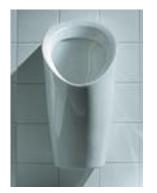
The LAUFEN Lema 0-litre urinal saves water and money. It operates without water and does not require a water shutoff device or electricity to keep the drain closed. The urine itself helps to keep gases sealed in and to prevent their escape. The principle behind this "trap" is known in the chemical industry as the Erlenmeyer flask.
