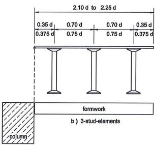
HALFEN HDB double headed studs for punching shear reinforcements
