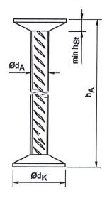
HDB studs identification on both (heads/ends) e.g.
