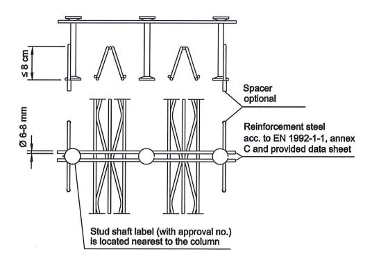
HALFEN HDB double headed studs for punching shear reinforcements
