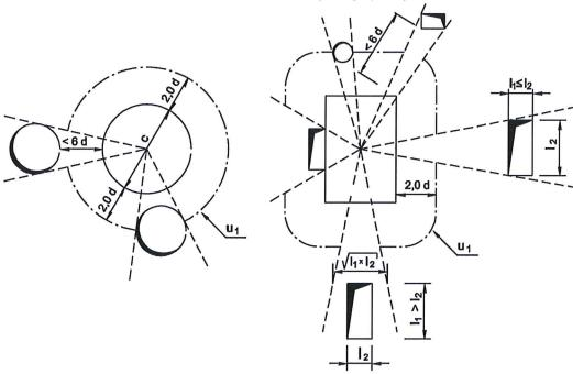
HALFEN HDB double headed studs for punching shear reinforcements
