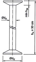
Material: reinforcement steel with a characteristic yield strength of  $f_{yk} \ge 500$  MPa acc. to EN 1992-1-1, annex C and provided data sheet
