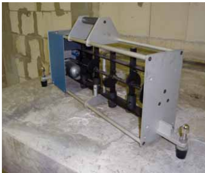
Standardised tapping machine according to EN ISO 10140
