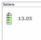
**Battery level indicator. In case of low battery, the color of the icon changes. A fully charged battery is comprised between 12.8 and 13.1V**
