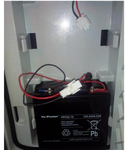
Their lifespan depends on the type of use. Autonomy with 1 single battery (without charge) is 3 to 8 days. Avoid moving Evolis Solution with batteries inside for security reasons and weight. If tricolor square is displayed (low battery warning), please replace both batteries with other charged.
