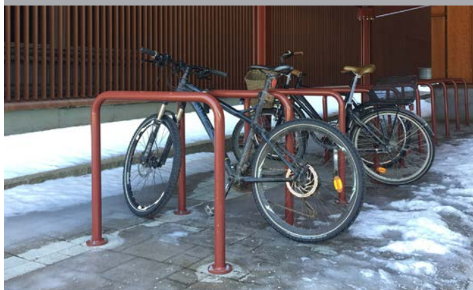
CYCLE STANDS DIAM. Ø48MM, POWDERCOATED
