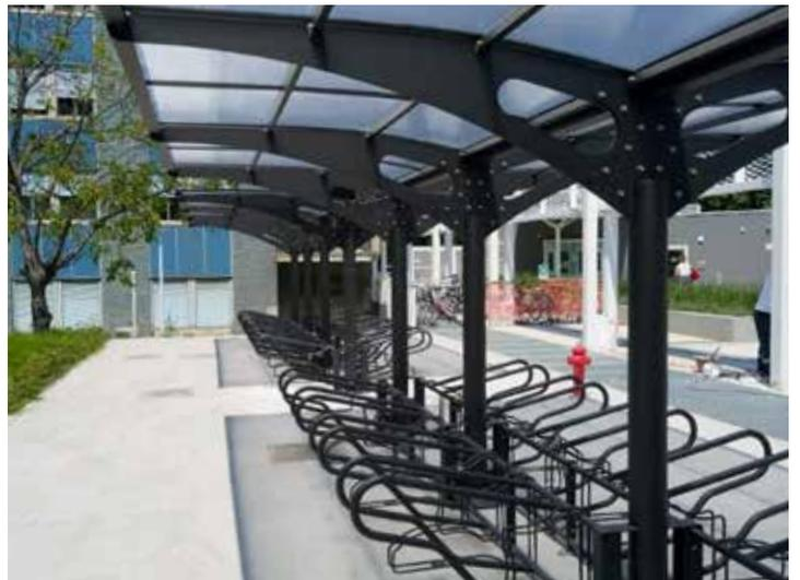
Cover double side made of two support in tubular steel and lateral sides of sheet. The cover could be in alveolar polycarbonate or in compact polycarbonate and it is supported by a tubular in steel. In the back of the cover there's a sheet gutter. The fixing at the ground is made with a circular plate with holes for the fixing with bolts. The bike rack (on request) is fixed on the supporting columns of the cover. All metal parts are galvanized and powder coated.
