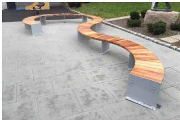
Bench with structure in galvanized and powder coated steel made up of supports in steel sheet with base plate for the fixing at the ground with bolts. The seat is made with wooden slats in natural pine wood treated for the external use. On request the wooden slats can be supplied in hardwood.
