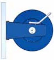
Hose guide installed outwards.
