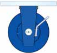
Hose guide installed outwards.
