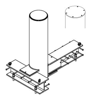
**Design:** Blocking bollard(s) with base supports for shallow mount installation. Bollard
