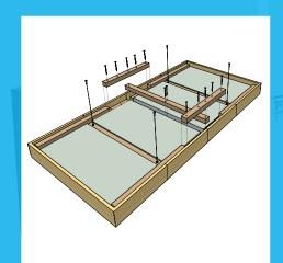
HERADESIGN® Sonic element 2400 is a 2400 x 1200mm acoustic ceiling raft with a unique HERADESIGN® Fine or HERADESIGN® Superfine surface.
