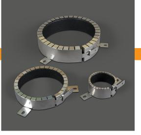
S&B Brandmanschett comprise of a range of devices designed to be fitted around plastic pipes or insulated metal and plastic pipes where they penetrate fire separating constructions. Under fire conditions the intumescent material within the collar expands to crush the softening pipe and/or combustible insulation, filling the resultant opening and maintaining the fire integrity and insulation performance of the floor or wall.
