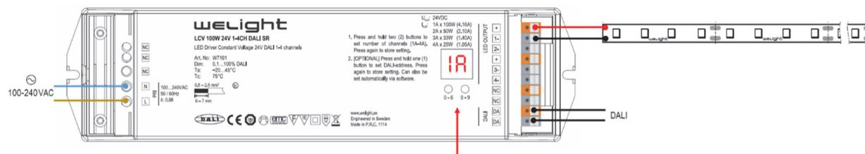
On later models (production batch  $\geq 1134$ ) the DALI terminals are located on the primary side (left):
