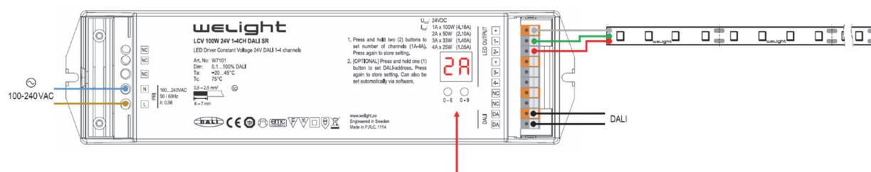
On later models (production batch  $\geq 1134$ ) the DALI terminals are located on the primary side (left):
