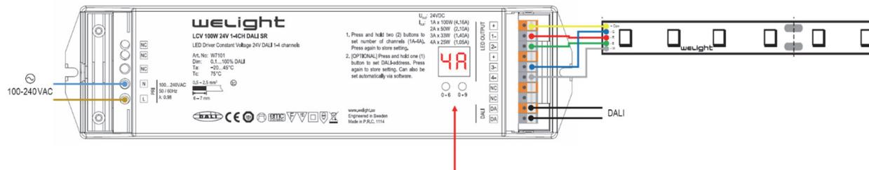
On later models (production batch  $\geq 1134$ ) the DALI terminals are located on the primary side (left):
