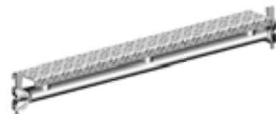
U-ledgers with gap cover, 0.11 m wide are available in a variety of lengths for gap-free work surfaces between U-main scaffolding decks and U-console bracket decks (see pages 42 / 43).
