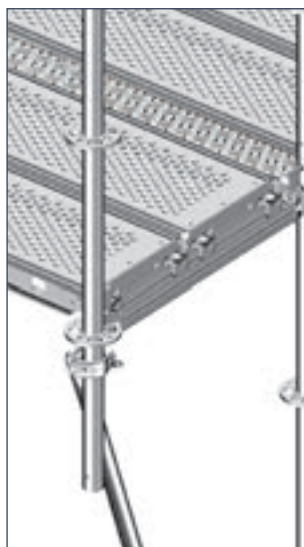
Assembly situation: U-console bracket, 0.73 m wide 3 (top) or alternatively U-ledger 0.73 m in conjunction with Bracket brace 2.05 m 10 (left).
