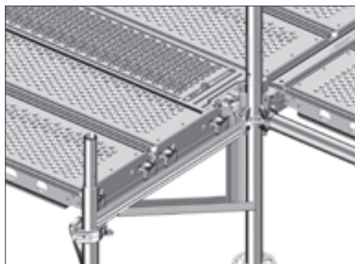
Assembly situation: U-console bracket, 0.73 m wide 3 (top) or alternatively U-ledger 0.73 m in conjunction with Bracket brace 2.05 m 10 (left).
