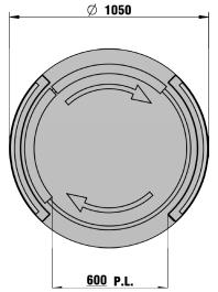
Concrete Base to specification at least (cube) 30N/mm2 of resistance. Base to be flat and level to  $\pm$ -5mm over footprint area. Dimensions to be > 1150 x 150 deep min. (units in mm).
