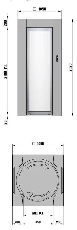
Concrete Base to specification at least (cube) 30N/mm2 of resistance. Base to be flat and level to +/-5mm over footprint area. Dimensions to be > 1150 x 1150 x 150 deep min. (units in mm).
