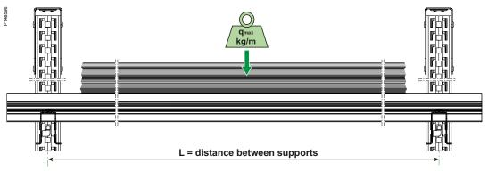
Ft (total load in N) = L (span or supports distance in meters) x qmax (load in kg/m) x 10.
