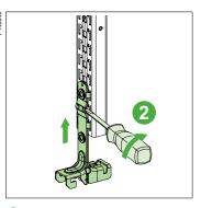
2 Twist the screwdriver to push the bracket upwards until the bracket is released.
