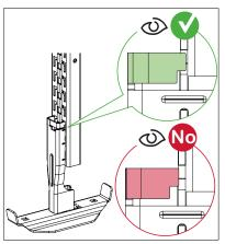
If the adapter needs to be reinstalled, correct the click lip to the initial position and make sure the click lip is locking properly.
