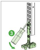
3 Use the screwdriver as a lever to pull down the bracket until the locking lip go inside the slot in the rail.
