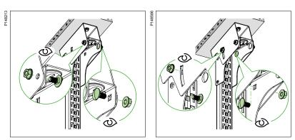
Fix the pendant to the adjustable ceiling plate with 4 bolt sets 22S and align the pendant to the vertical plane before tightening the bolts. Recommended torque 20 N.m.
