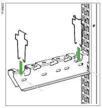
2 fast fixing clamps are required per cantilever.
