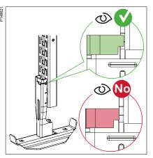
Visually check and secure that the adaptor is properly positioned, and the click lip is properly positioned inside of the slot of the CLX<sup>3</sup> rail.
