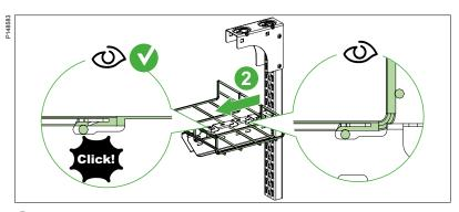
2 Pull the mesh tray horizontally towards the tip of the cantilever arm until the mesh tray wire passes the locking lip and clicks into position.
