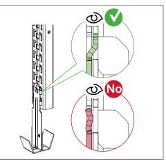
Visually check and secure that the bracket is properly positioned, and the click lip is positioned inside the slot in the CLX<sup>3</sup> rail.
