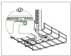
Visually check that the wire is properly positioned and the wire has passed the locking lip.
