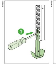
Fit the head of screwdriver on the side of the locking lip.
