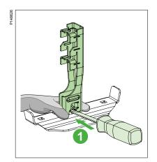
• Hold the bracket, fit the screwdriver's head between the adaptor lip and the bracket.
