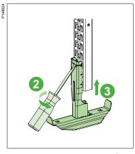
Use the screwdriver as a lever to 2 gently release the click lip from the rail. Then 3 push the adaptor up to release the L hooks from the rail.
