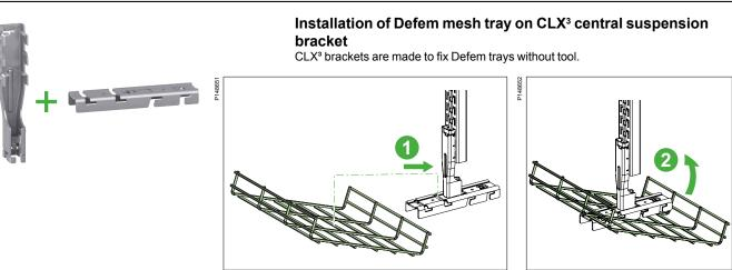
**(**) Slide the middle of the mesh tray on the upper slot side of the bracket and insert the longitudinal wire on the most center top slot.
