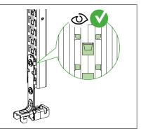
Visually check and secure that the cantilever arm is properly positioned and the locking lip is positioned inside of the slot in the CLX<sup>3</sup> rail.
