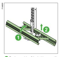
Push one side of the ladder up until the ladder leave the lip of the bracket.
