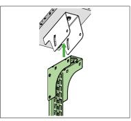
Insert the pendant into the adjustable ceiling plate.
