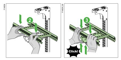
2 Squeeze the free side of the ladder strongly down on the outer end of the cantilever until 3 the ladder overpasses the locking lip.
