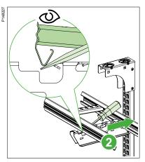
After releasing the outer side of the ladder, 2 push the ladder in the direction of the rail to unlock the other side.
