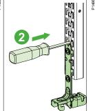
Hold the bracket and 2 insert the screwdriver in the slot just above the bracket.
