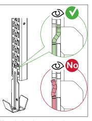
When the bracket needs to be reinstalled, correct the click lip to the initial position and make sure the click lip is locking properly.
