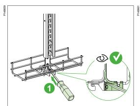
Uninstallation of Defem mesh tray from CLX<sup>3</sup> Defem central suspension bracket 120/220
