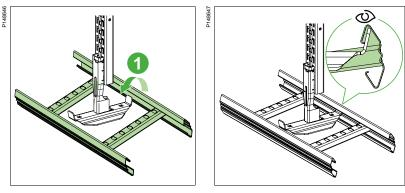
1 Insert one inside side of the ladder on one lips of the bracket.
