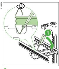
Fit the head of the screwdriver between the ladder and the top surface of the cantilever as in the picture. Use the screwdriver as a lever to pull out the ladder of the locking lip until the ladder snaps out.
