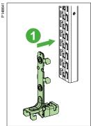
• Press the bracket until the hooks are fully inserted in the pattern and the surface touches the rail.
