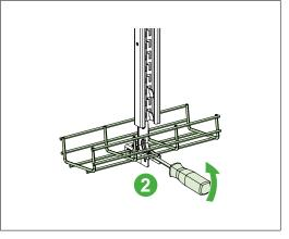
Hold the bracket and 2 use the screwdriver as a lever until the mesh tray overpass the locking lip.
