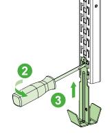
2 Use the screwdriver as a lever to gently bend the lip. 3 Push the bracket upwards.
