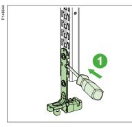
(1) Insert the head of the screwdriver in the bump in the bracket and with the head simultaneously gripping in one of the slots in the rail.
