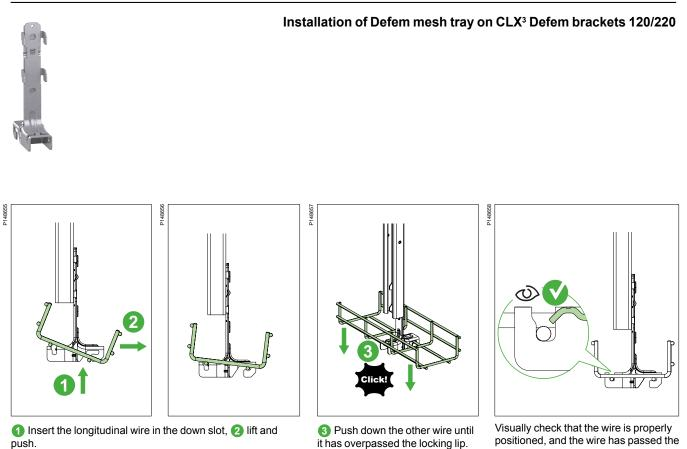
positioned, and the wire has passed the locking lip.
