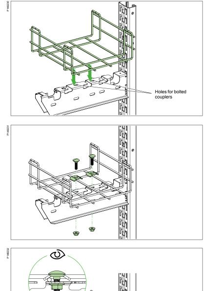
Place the Performa mesh tray on the top surface of the cantilever arm, as close as possible to the rail and by leaving at least 20 mm.
