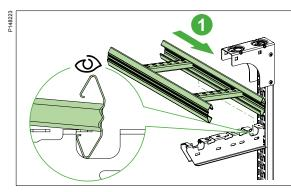
(1) Insert the ladder on the rail side. Pull it on the outside direction to lock this side in the lip.
