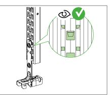
Visually check and secure that the bracket is properly positioned, and the click lip is positioned inside the slot in the CLX<sup>3</sup> rail.
