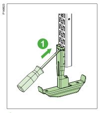
1 Fit the screwdriver's head in the slot of the adaptor.
