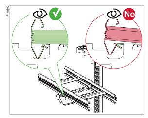
Visually check that the ladder is properly positioned, and the locking lip is positioned inside of the ladder profile.
