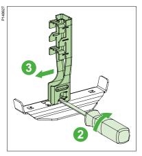
2 Twist the screwdriver to use it as a lever on the click lip until it passes over the bracket's locking lip and 3 pull the adaptor sideways to release it.
