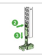
Press against the top of the bracket towards the rail and 3 pull it down until the locking lip go inside the slot in the rail.
