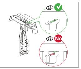
1 Insert the adaptor in the pattern on the central suspension bracket.
