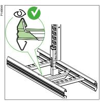
Visually check if the bracket lip is inside the ladder profile. Profile clamp 43 can be used to fix the cable ladder to the support bracket.
