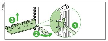
Fit the head of the screwdriver between the rail and the locking lip of the cantilever.
