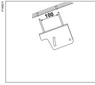
Fix the adjustable ceiling plate to the ceiling with 2 bolts. (c-c: 100 mm).
