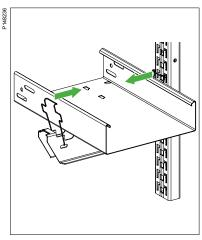
Fix the top of the spring on the top of the tray.
