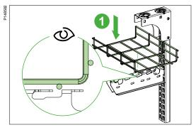
1 Insert the longitudinal wires in the slots.
