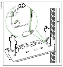
Place the hooks of the clips in the holes on the side of the  $CLX^3$  cantilever arm at the appropriate width for the tray to be fixed.
